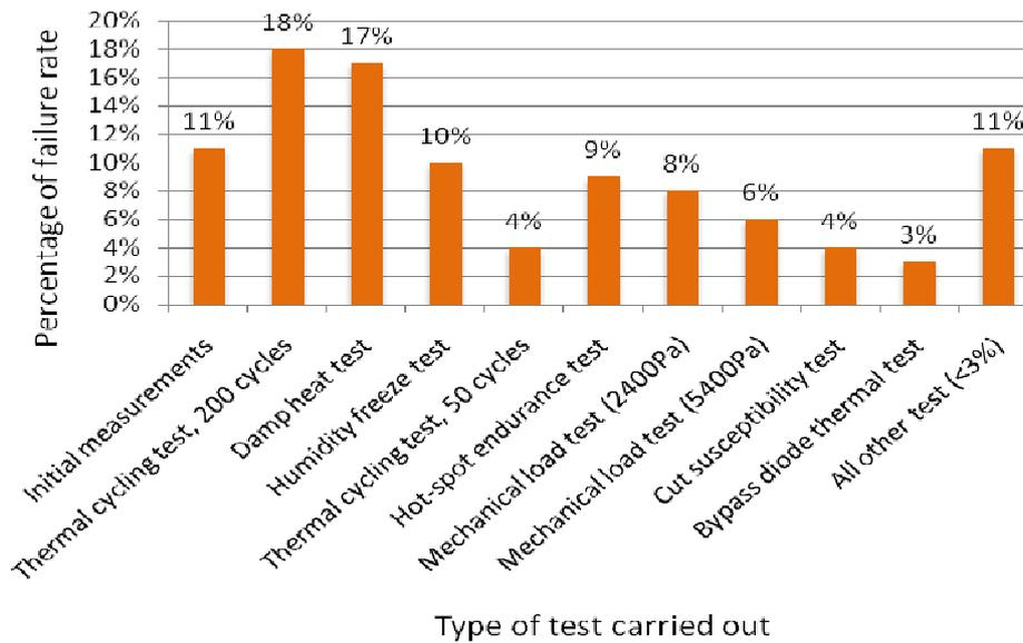
**Figure 12: Distribution of Failed Tests of 1740 IEC Projects**
