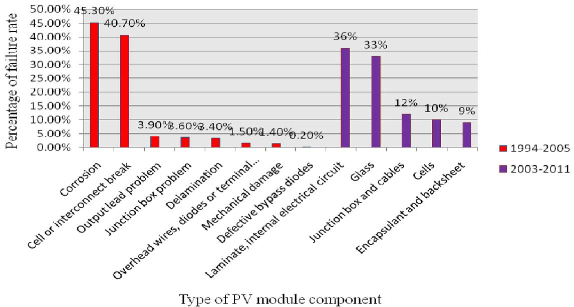
**Figure 13: Types of PV Module Field Failures Observed**
