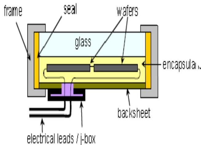
**Figure 10: Typical Packaging of Crystalline Silicon PV Module [1]**
